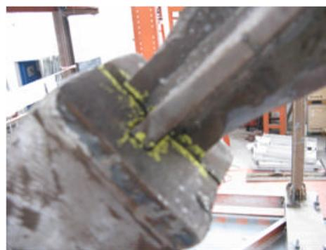
*(a) Status of the buckling restrained brace before test*
