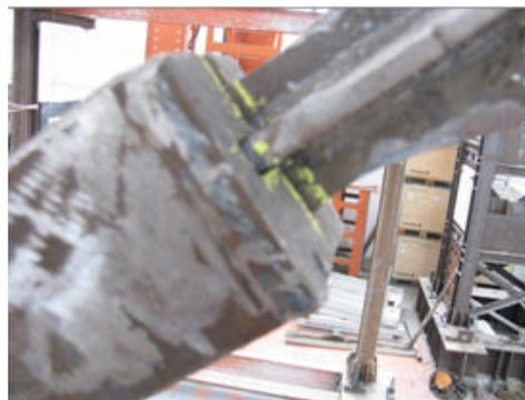
*(b) Status of the buckling restrained brace after test*
