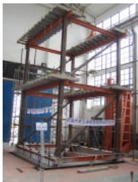
*Shaking table test on a steel frame with semi-rigid composite connections and buckling restrained braces*
